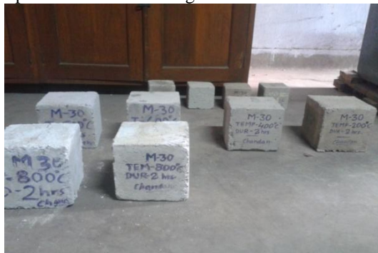
Figure 3.2 concrete cube at different elevated temperature
