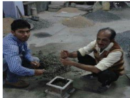
Figure (2.2) compaction of concrete manually.
