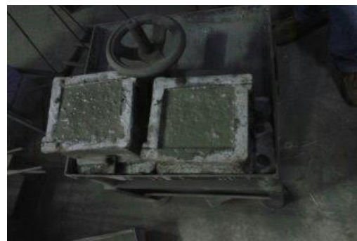
Figure(2.3) Compaction on vibrating table.
